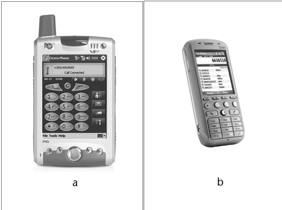
Figure 15.8 SIP user agent for GSM- and Wi-Fi-enabled PDA (courtesy Cicero Networks). (a) HP PDA, (b) Qtek mobile phone
