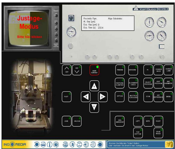
Fig. 1 The real mask aligner MA6 (top) and its virtual pendant, the computer based training tool (bottom)
